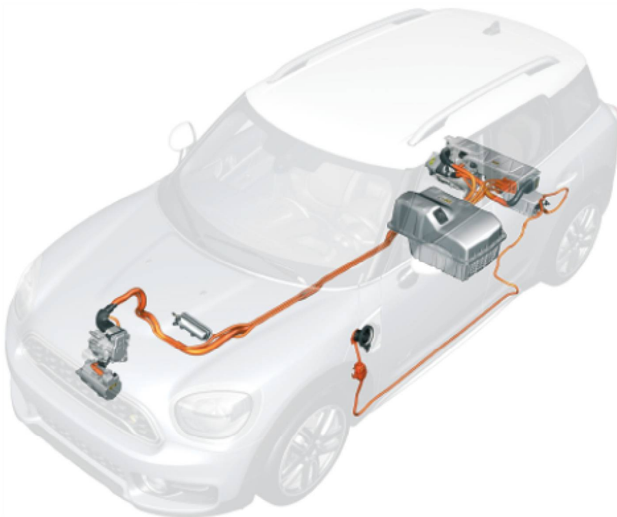
Position of the high-voltage components
