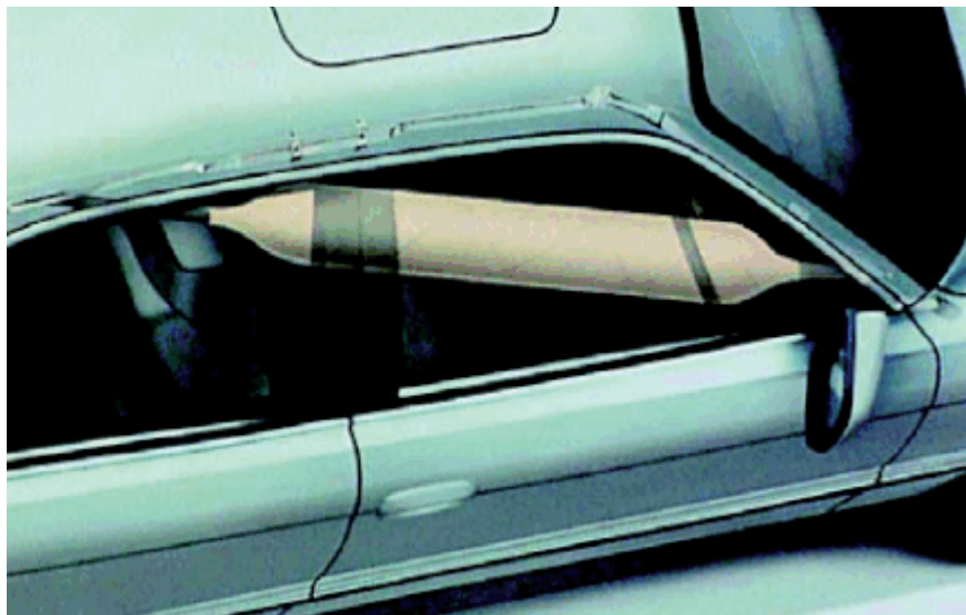
Inflatable tubular structure not activated (in the roof area) and activated
