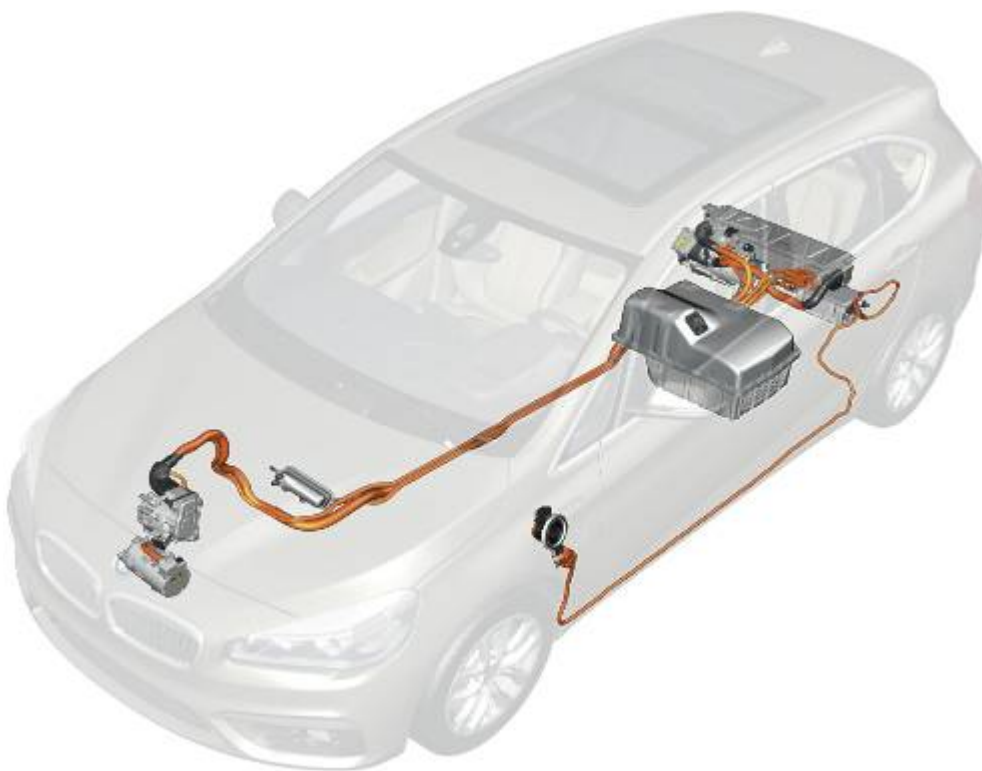
Position of the high-voltage components
