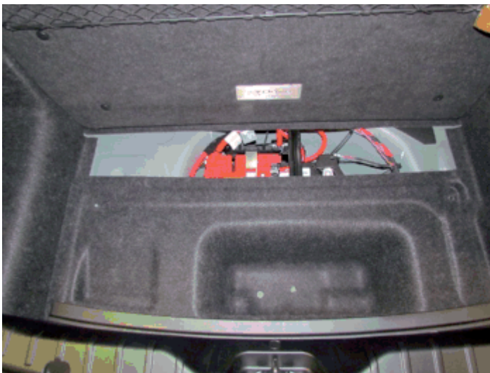
Installation positions of the 12 V batteries
