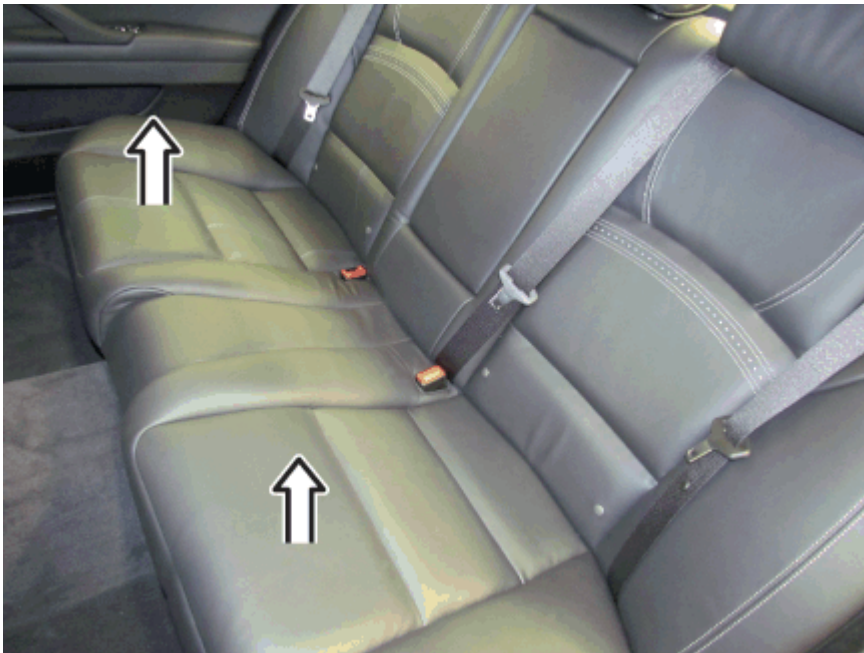
6. Disassemble the rear seat bench by the reaching underneath and pulling firmly.
